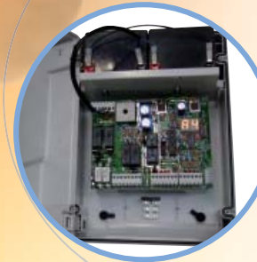
ENCLOSURE FOR CONTROL UNITS | page 11 TO HOUSE ALL THE RANGE OF THE 24V GENIUS CONTROL UNITS
